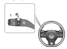
With the START/STOP Switch in the ON/READY position and the headlamps on, rotate the fog lamp switch to position I to turn on the rear fog lamp. The rear fog lamp indicator illuminates in the instrument pack when the rear fog lamps are on.
