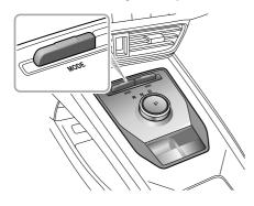
The driver can select three driving modes by operating the MODE switch:
