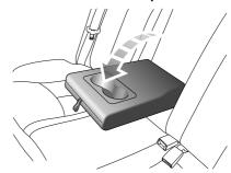
Fold forward to open the rear armrest. There are cup holders at the front end of the rear armrest.
