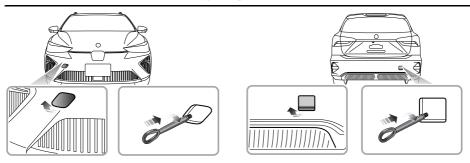
Your car is equipped with 2 towing eyes (located at the front and the rear of the vehicle), which are used for fitting the towing hook in the tool kit. The tool kit is placed beneath the loadspace floor.
