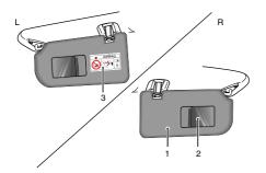
Note: Warnings and instructions on use of child restraint (3) are attached to both sides of the passenger sunvisor.
