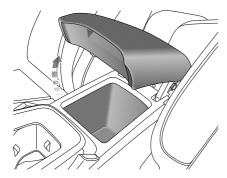
Lift the armrest (arrowed) to open the compartment cover and put down to close.
