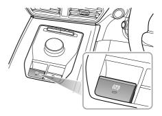
The EPB can be applied and released in two ways:
