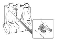
To increase the luggage space, the rear seat backrest can be folded fully forward. When folding the backrest completely, firstly insert the rear seat belt buckle into the corresponding slot, then fully lower (or remove) all head restraints, pull the respective control lever at the top of the seat backrest upwards and fold the seat backrest forward.
