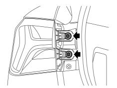
4 Release the tail lamp assembly and disconnect the connector.
