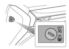
The passenger airbag switch is located in the left fascia panel end cover trim. Insert the key and rotate the switch to the on or off position to enable or disable the passenger airbag.
