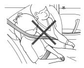
As children grow and become older/larger it will get to the stage when they no longer require child seat restraints, at this point they will require use of the vehicle standard seat belt. Please ensure the seat belt is correctly positioned on the body of the child.
