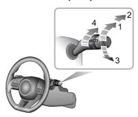
The rear wiper and washer will only operate when the START/STOP Switch is in the ON/READY position. Rotate the rear window wiper switch to your desired selection:
