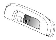
The rear interior lamps are located on the left and right sides of interior roof panel. Press the lamp lens as indicated in the diagram to switch on the rear interior lamps, press it again to switch off the lamps.
