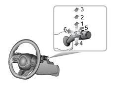
The front wipers and washers will only operate when the START/STOP Switch is in the ON/READY position. Operate the stalk switch to select different wiping modes:
