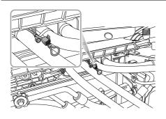
Pull the release cable handle, remove the connector plug whilst maintaining tension on the cable this will release the locking device.
