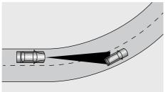
When turning at an intersection or following a vehicle into, or out of a curve, the adaptive cruise control system may be unable to detect the vehicle ahead, even if it is in the same lane, it is possible the system may detect a vehicle in another lane.
