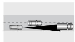
If the vehicle ahead changes lanes, but does not drive into the lane completely, the adaptive cruise control system may be unable to detect the vehicle.
