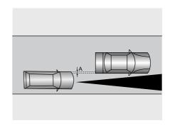
When driving behind a vehicle that is only partially overlapping your vehicle, 'A' in the graphic, the adaptive cruise control system may be unable to detect anything.
