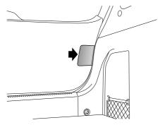
3 Rotate the reverse lamp holder in counter-clockwise and remove the holder and bulb.
