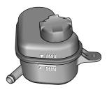
The cooling system should be checked weekly when the cooling system is cold and with the car resting on level ground. If the coolant level is below the "MIN" mark, open the coolant expansion tank cap and top up coolant. The coolant level should not be higher than the "MAX" mark.
