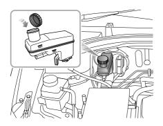
Note: Brake fluid can damage painted surfaces. If you accidentally spill the brake fluid on the painted surface, soak up any spillage with an absorbent cloth immediately and wash the area with water or car shampoo.
