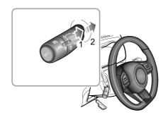
The traffic jam assist system switch is located in the infotainment display. Enter the corresponding interface for driving assistance to turn the system ON/OFF. Operating the adaptive cruise control level to "RESUME" twice will switch the traffic jam assist system to standby or active state.
